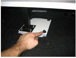
Attach assembly to vehicle using OEM seat hardware and nutcerts in vehicle
